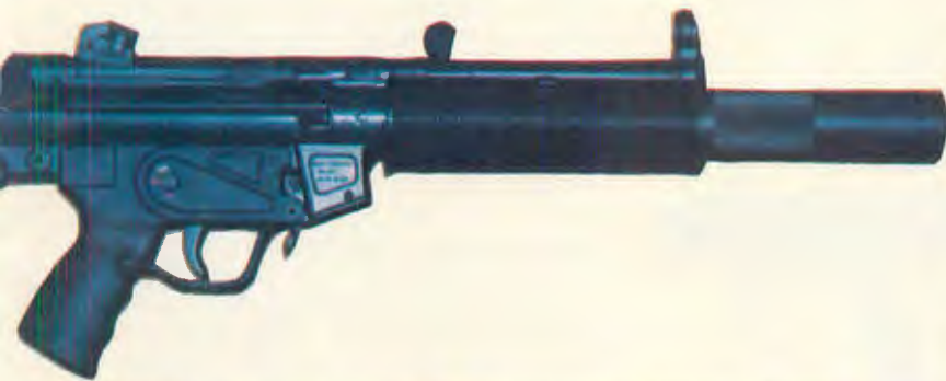
MP5 SD A3 submachine gun features telescoping stock and suppressor. Vent holes bleed off gas right out of chamber which prevents 9mmP bullet from exceeding supersonic velocities, thus eliminating muzzle blast and sonic "crack."
